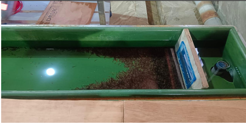
Figure 9. Fish were swept away towards the outlet by excess water flow
